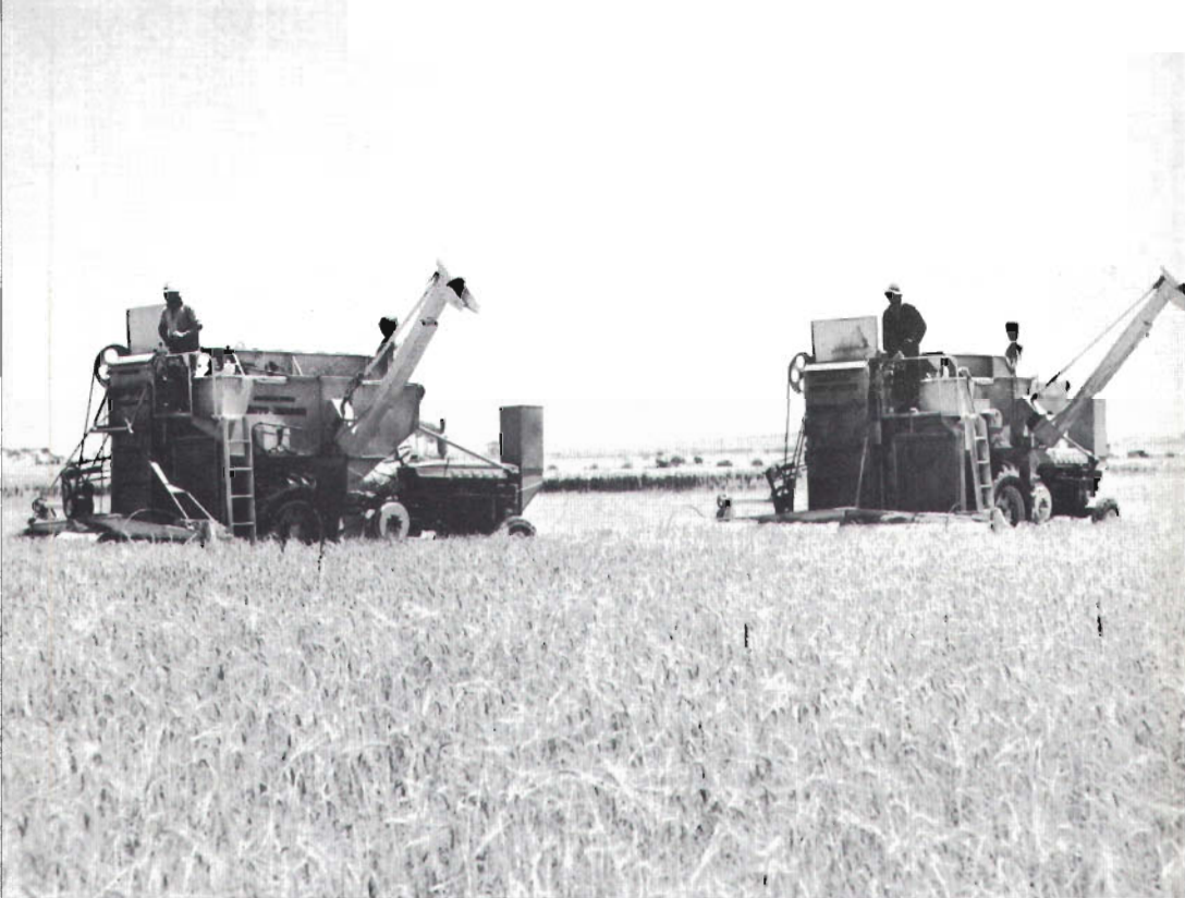
Harvesting wheat in the Wimmera. These self-propelled headers each harvest a 16 ft strip, store the grain in a bin, and transfer it to trucks through their elevators.
